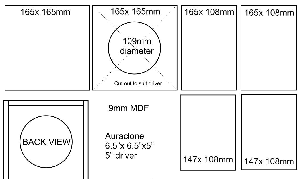
Glued with PVA, internal edges with 10x10mm timber bracing
